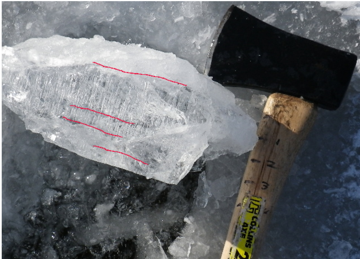
Chopped block of ice shows distinct layers created by fluctuating temps. Ice is about 4 inches thick with a 3 inch layer of black ice which is full of air bubbles. The black ice in this sample is not as strong as hard clear ice. If temps rose above freezing this ice would get weak quicker than the harder clear stuff. Lake Lee, Kodiak, AK
