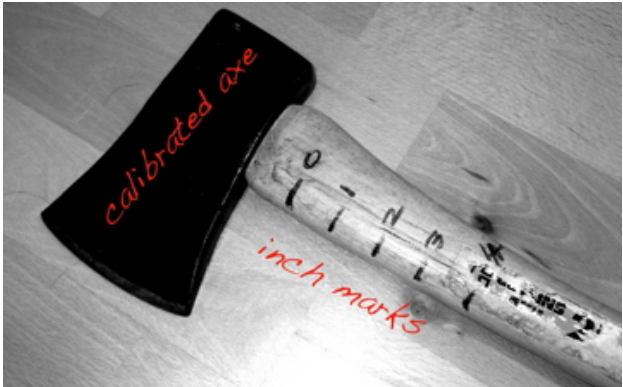
Calibrated axe. The axe can be drawn up against the underside of an ice sheet through a chopped hole. Zero allows for curve of axe head and a safety factor.
