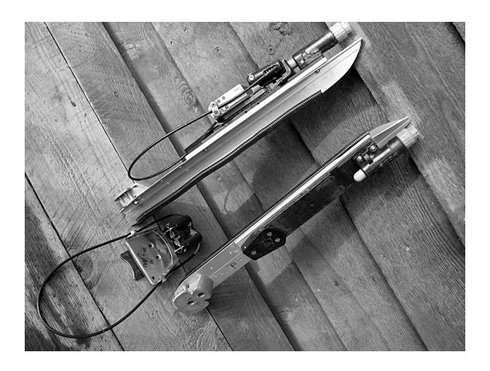
Here are 55cm nordic skates with a wide deck. The adapter plate is 1/4" 6061 T6 and allows for the Viole (Americana Besser Plate style) piston to be mounted forward. Bindings shown are telemark.
