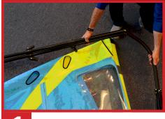
Insert front tubes to sleeves in sail. Brackets on front tube align with holes in sail.
