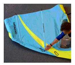
Fold the sail with bracket holes visible.
