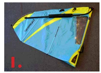
2. Stow battens, cross tube and tip wands. Stow battens so they are protected by the boom with the curved ends of battens next to curved end of boom.
